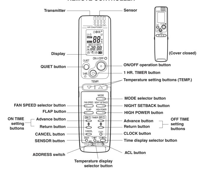
**NOTE** The illustration above pictures the remote controller after the cover has been opened.
